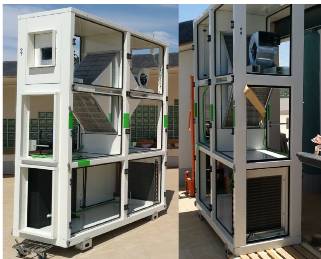
Fig. 7. Prototype air conditioning system structure.
